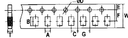
12.2 Dimension of plastic taping: (Unit: mm)
